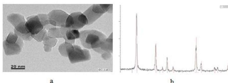
Figure 1: Characterization of TiO<sub>2</sub> nanoparticles: A: SEM image of TiO<sub>2</sub>-NPs, B: X-ray image of TiO<sub>2</sub>-NPs.
